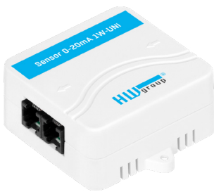
Sensor 0-20mA 1W-UNI 8-point calibration table
