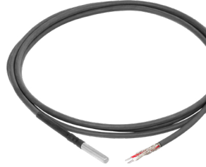
Probe Pt100 TG8 2 m Temperature range: -50 to 200 °C, IP67 rating
