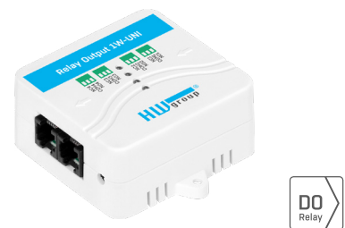
Relay Output 1W-UNI 4x relay output, supported only by HWg-Ares12 and Ares 12 LTE
