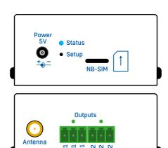
A module with 2 relay outputs controlled from the SensDesk portal over the NB-IoT network. To reduce consumption, the device features two latching relays. For increased reliability, the relays are energized repeatedly every 10 minutes. The device is not suitable for mobile applications. On battery power only, the estimated battery life are 2 years.
