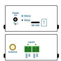
A device for connecting a door or window contact, a PIR motion detector or a smoke or gas detector with a dry contact output. Allows connecting 2 independent detectors. Inputs feature pulse counters for connecting energy meters with an SO output. **Due to high energy requirements of SO outputs, external power is required for reliable pulse counting.** Otherwise, reliable operation cannot be guaranteed.
