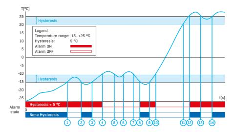
The figure demonstrates two cases. Without the hysteresis idle range of 5 °C, the alarm raised in point 8 would end in point 9; however, the hysteresis function keeps the alarm active until the temperature reaches the upper limit of the tolerance band (point 10): 5 °C + (-15 °C) = -10 °C.
