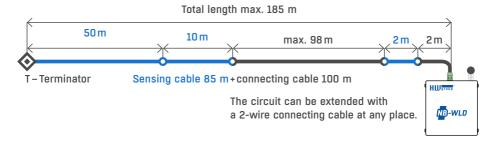
The flood detection is performed every 5 minutes and the estimated battery life are 4 years. If the cable is flooded or disconnected and the device is powered from an external adapter, the red LED lights up. The LED is inactive on battery power.
