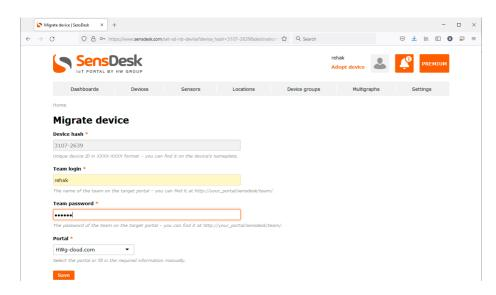
After you click the **Save** button on the web page, take a pencil or other tool and briefly **press the Setup button on the device**. It will start blinking (communication with the portal) and finalize the device migration process.
