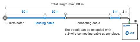
Flood detection is performed every 5 min. (15 min. when powered from the battery). Estimated battery life with 15 min. detection is 4 years.
