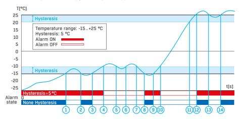
The figure demonstrates two cases. Without the hysteresis idle range of 5 °C, the alarm raised in point 8 would end in point 9; however, the hysteresis function keeps the alarm active until the temperature reaches the upper limit of the tolerance band (point 10): 5 °C + (-15 °C) = -10 °C.
