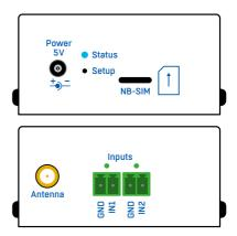
Remote monitoring device for connecting external detectors to 2x DI (Digital Input). To each DI input you can connect a door or window contact, a PIR motion detector or a smoke/gas detector with a dry contact (relay) output.
