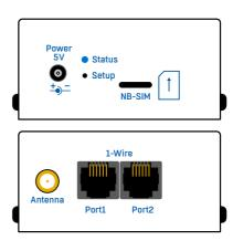
A device for connecting external sensors of Temperature, Relative Humidity, Voltage or other values via the RJ11 1-Wire (UNI) bus. 2 RJ11 ports allows connecting several external physical sensors to measure up to 4 sensor values simultaneously.
