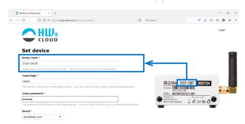
Setting up the device IoT Monitoring
